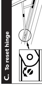
Adjust friction screw in green slider to allow for smooth operation of the hinge
