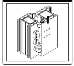
4 Ensure the adjuster sledge screw is flush with the edge of the sledge
