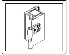
7 Fit sash to frame and fix cover with the screws (included)
