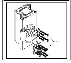
6 Press compression bush into body with alignment mark facing away from the sash
