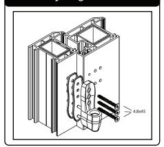
3 Locate peg into slot and firmly push hinge into the body
