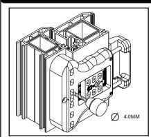
2 Add packers if required & fix body using 3x 45mm screws
