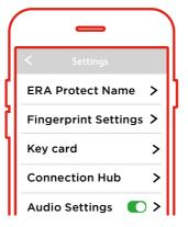
To turn on Audio, repeat the steps and slide the button to the right. A pop up box will confirm audio is now enabled.
