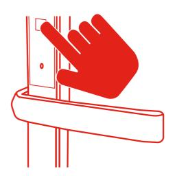
Using your chosen fingerprint (finger / thumb), place over the black sensor on the front of the external handle.
