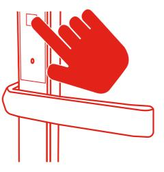
Follow the steps provided by the "voice prompt". Once complete, please test to see if the added print can successfully open the door. Close the app and place the stored print on the ERA Protect handle. You will hear "door open" (if voice is enabled) and you can push the handle down to unlock.
