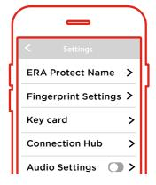
Using the slider next to "Audio Settings" you can turn on and off. Audio is turned "on" by default. A pop box will confirm audio is disabled.
