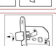
tool provided; insert the tool behind the shoulder of the latch shaft as shown and rotate the bolt head 180°.
